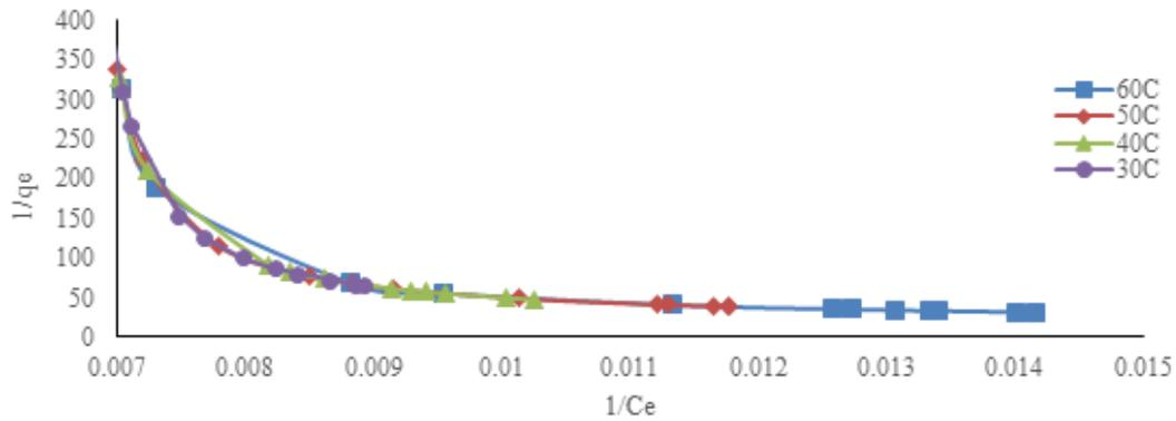
**Figure 9.** Langmuir adsorption isotherm for chromium (VI)-*P. aeruginosa* ANSC dried biomass system: temperature = 30-60°C; pH 2; biomass = 1 g; time = 2 h
