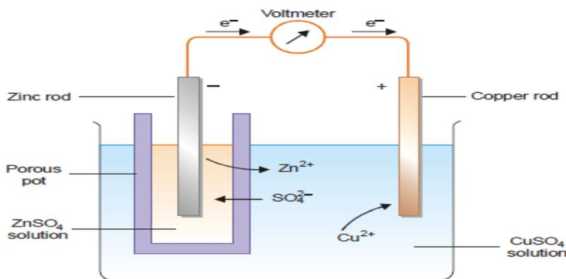
In this cell the salt-bridge has been replaced by a porous pot. Daniel cell resembles the above voltaic cell in all details except that  $\text{Zn}^{2+}$  ions and  $\text{SO}_4^{2-}$  ions flow to the cathode and the anode respectively through the porous pot instead of through the salt-bridge. In spite of this difference, the cell diagram remains the same.
