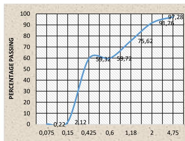
Fig. 8. Particle Size Graph on a Fine Sand
