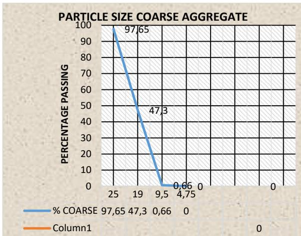
Fig. 9. Particle Size Graph on a Coarse Aggregate
