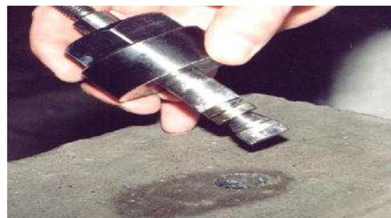
Fig. 6. The expansion unit inserted in the hole and capo-insert fully expanded to 25 mm diameter
