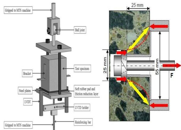
Fig. 4 and Fig. 5. Schematic of Pullout test apparatus
