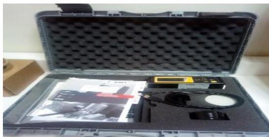
Fig. 2. Concrete Test Hammer Kit
