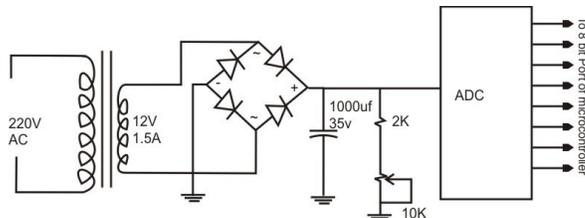
Figure 4 Voltage Detector
