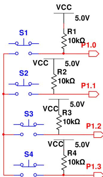
Figure 3 Circuit Implementation of Mode Select Switches
