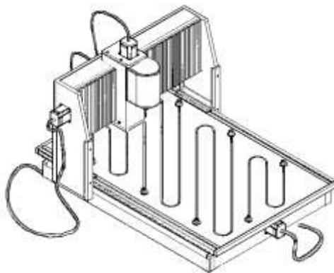
Figure 1: 2D Wireframe drawing of the proposed Router
