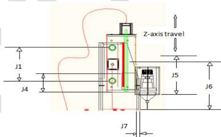
Figure 3: Side view of the Z-axis assembly
