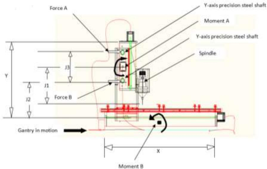
Figure 2: Analysis of the Y-axis assembly Parameters
