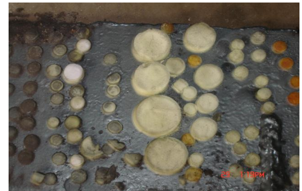
Plate 2: ZnO varistor samples cooling down to room temperature after sintering.
