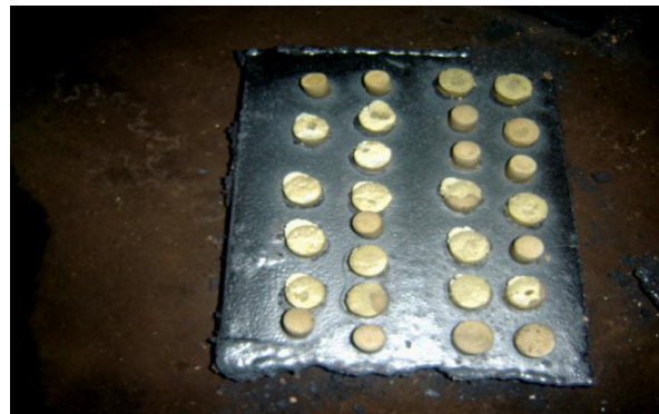
Plate 1: Samples Of ZnO Varistors Disc Pellet Ready For Sintering.
