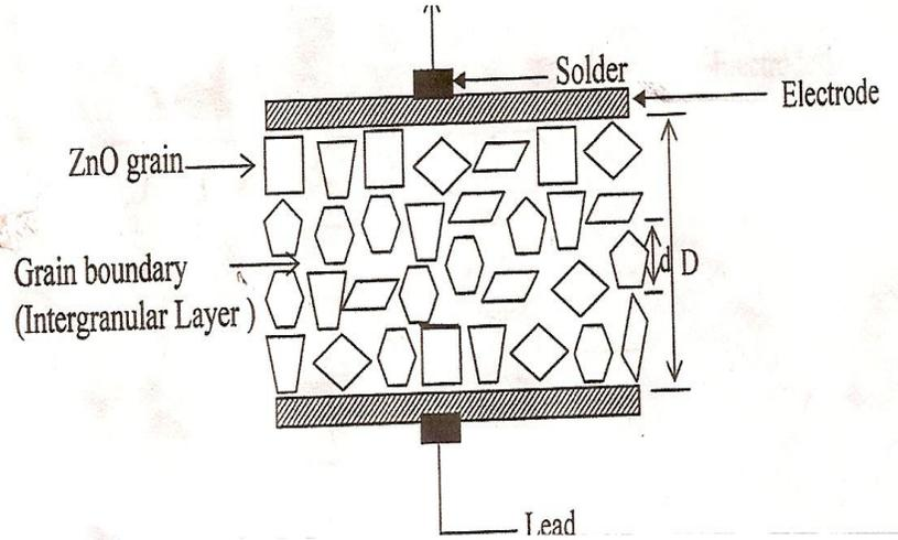
Figure 1. The schematic diagram of zinc oxide varistor
