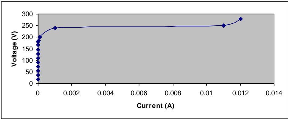
Fig.3; V-I Characteristics of ZnO varistor (Sample 2)
