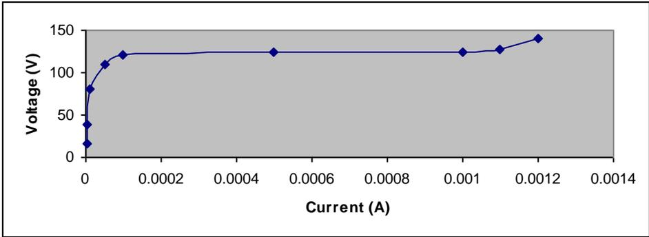
Fig. 2; V-I Characteristics of ZnO varistor (Sample 1)
