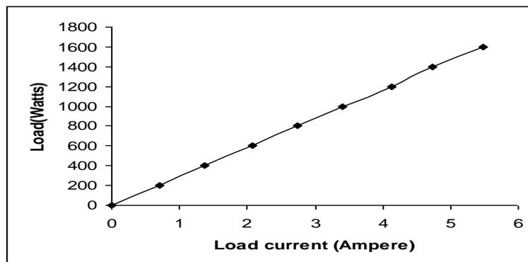
Figure 2 Load-current characteristics of 1.4kW, 220V, 50Hz inverter.
