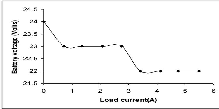
Figure3 Effect of load current on the terminal voltage of the battery.
