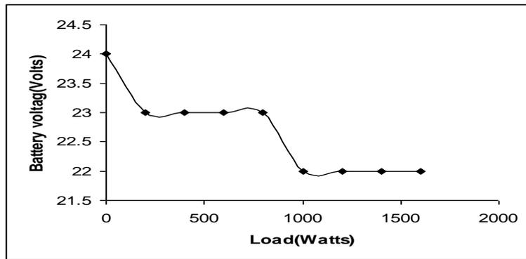
Figure 1 Effect of load on the terminal voltage of the battery.
