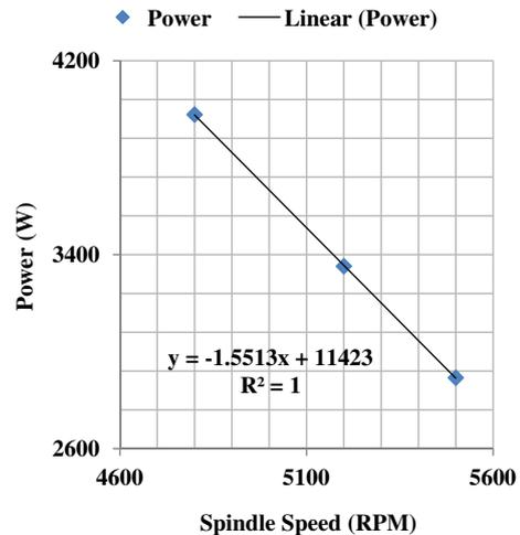
Fig. 9. MAC-V2 Takisawa Milling Machine no load power-spindle speed characteristic in zone C to 5500 rpm.
