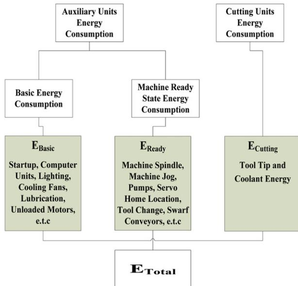
Fig. 1. Machine tool electrical energy consumption estimation model.
