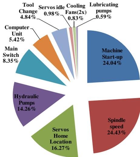
Fig. 3. Non-cutting power consumption distribution of the MHP MDSI CNC open lathe machine.
