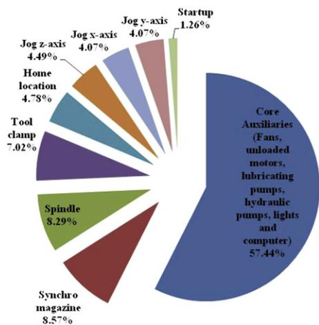
Fig. 4. MAC-V2 Takisawa Milling Machine auxiliary units power demand.
