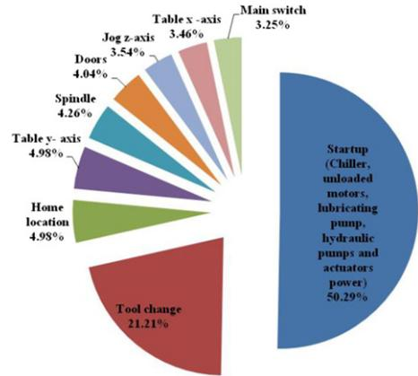
Fig. 5. Mikron HSM 400 high speed machining, auxiliary units power demand.
