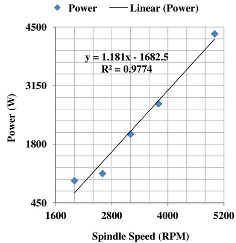
Fig. 8. MAC-V2 Takisawa Milling Machine no load power-spindle speed characteristic in zone B to 5000 rpm.
