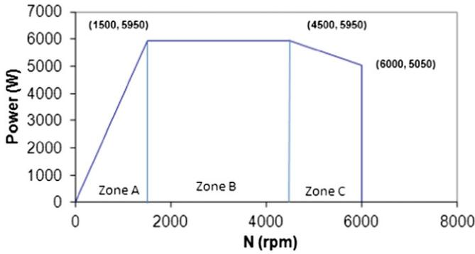
Fig. 6. Power-speed characteristics of a MAC-V2 Takisawa Milling Machine tool and 3 zones for energy profile.
