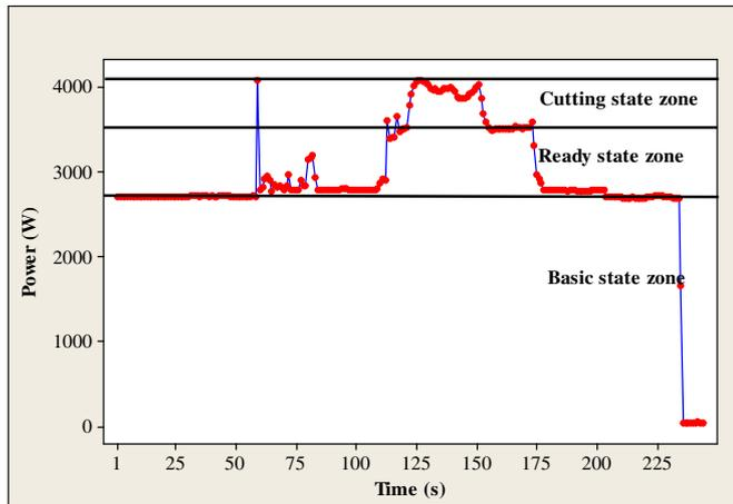
Fig. 10. Total power consumption trend for machining toolpaths.
