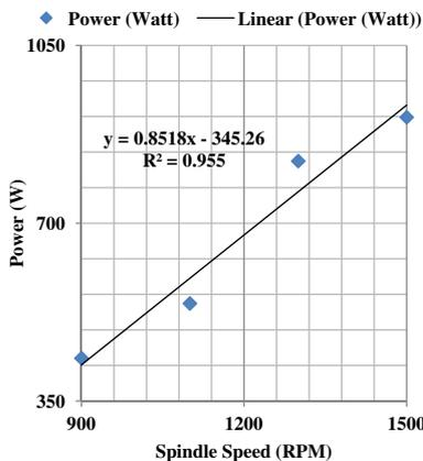
Fig. 7. MAC-V2 Takisawa Milling Machine no load power-spindle speed characteristic in zone A to 1500 rpm.
