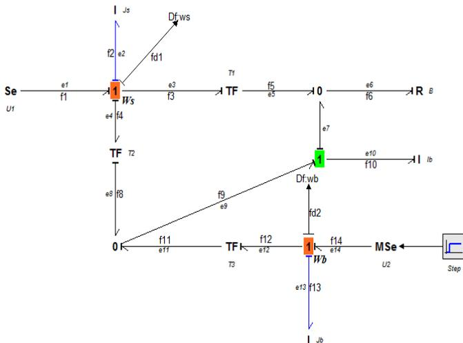
Fig. 9: Observability Analysis of the Ball-on-Sphere System Preferential Derivative Causality
