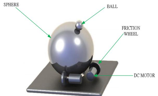
Fig. 1: Ball on a Sphere System [1]
