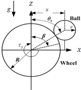
Fig. 4: Ball and Wheel System in x-axis [6]
