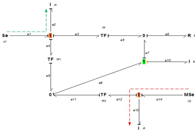
Fig. 6: Controllability Analysis of the Bond-on-Sphere System Bond Graph Model with Preferential Integral Causality
