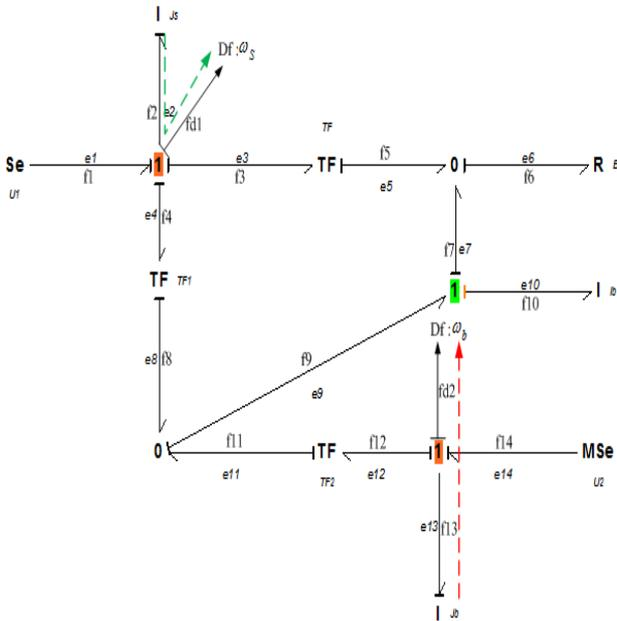
Fig. 8: Observability Analysis of the Ball-on-Sphere System Bond Graph Model with Preferential Integral Causality
