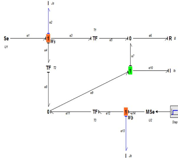
Fig. 7: Controllability Analysis of the Ball-on-Sphere System Bond Graph Model with Preferential Derivative Causality
