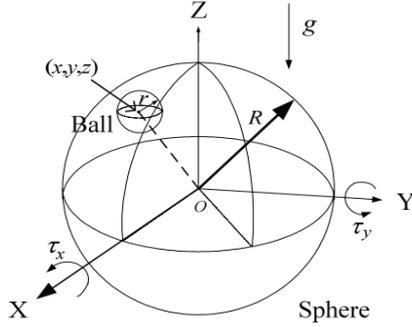
Fig. 3: Ball-on-Sphere System[6].
