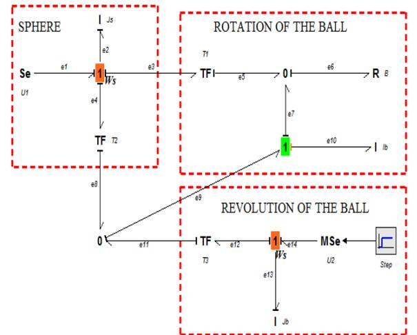
Fig. 5: Causal Bond Graph Model of the Ball-on-Sphere System [16]
