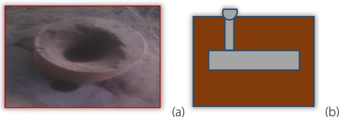
Figure 1. Casting of samples in sand moulds
