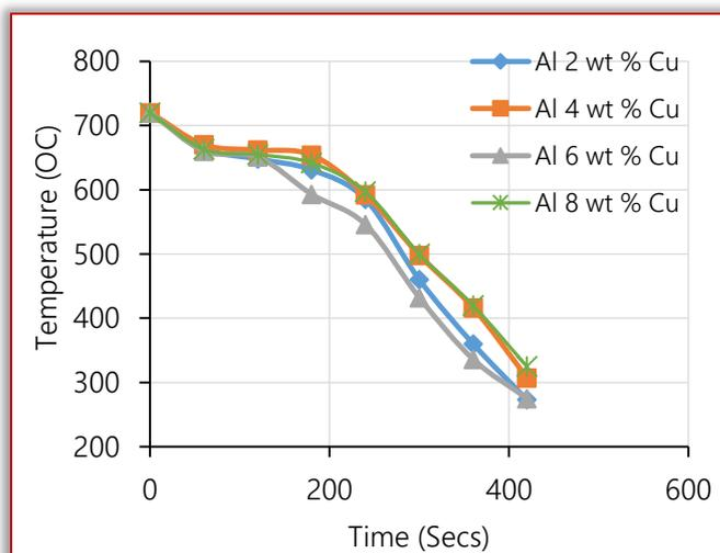
Figure 2: Cooling curves for Al-Cu alloy
