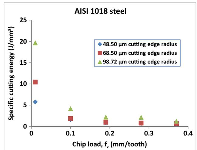
**Fig. 7** Variation of specific cutting energy with chip load during side milling of AISI 1018 steel with different cutting edge radii
