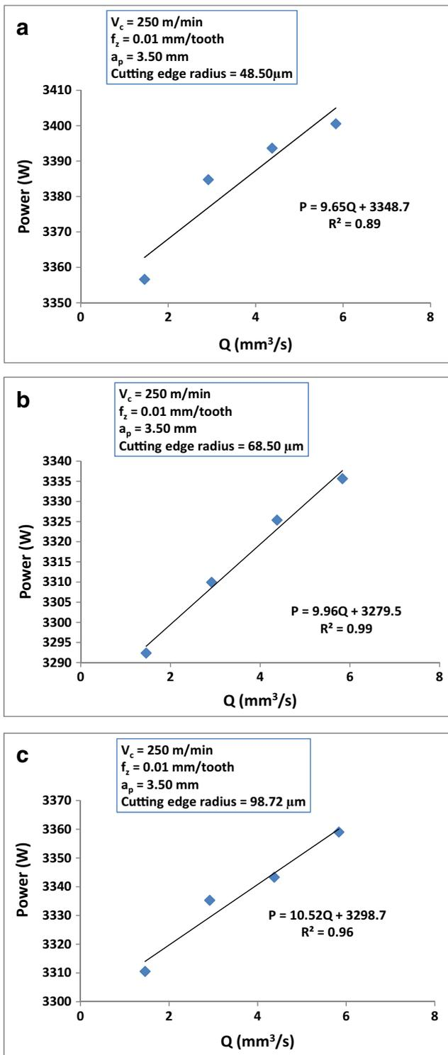
**Fig. 4** a Power\_MRR during side milling of aluminium AW6082-T6 alloy using  $48.50 \mu\text{m}$  cutting edge radius insert. b Power\_material removal rate (MRR) during side milling of aluminium AW6082-T6 alloy using  $68.50 \mu\text{m}$  cutting edge radius insert. c Power\_material removal rate (MRR) during side milling of aluminium AW6082-T6 alloy using  $98.72 \mu\text{m}$  cutting edge radius insert
