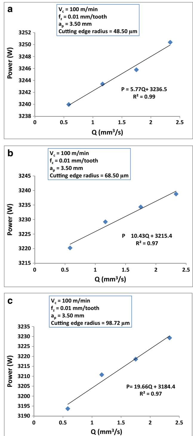
**Fig. 5** a Power\_material removal rate (MRR) during side milling of AISI 1018 steel using  $48.50 \mu\text{m}$  cutting edge radius insert. b Power\_material removal rate (MRR) during side milling of AISI 1018 steel using  $68.50 \mu\text{m}$  cutting edge radius insert. c Power\_material removal rate (MRR) during side milling of AISI 1018 steel using  $98.72 \mu\text{m}$  cutting edge radius insert
