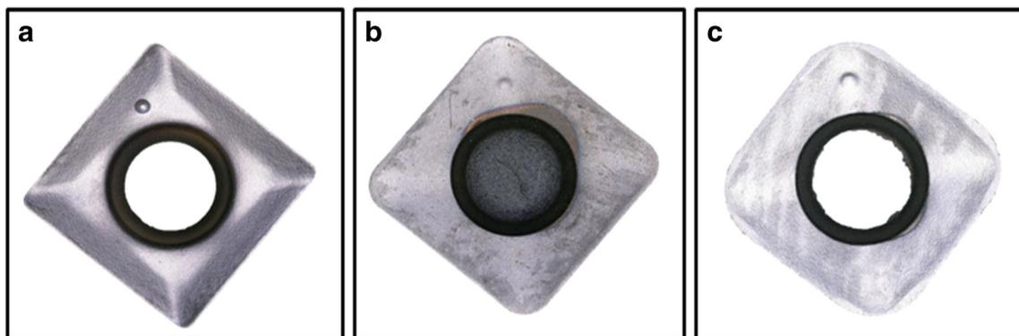
Fig. 1 a Iscar SOMT-060204-HQ IC328. b Iscar SOMT-060208TN-HQ IC328. c Iscar SOMT 060216TN-HQ IC328
