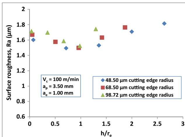
**Fig. 9** Variation of surface roughness with ratio of undeformed chip thickness to cutting edge radius during side milling of AISI 1018 steel using different nose radii of insert
