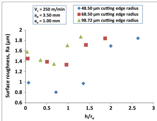
**Fig. 8** Variation of surface roughness with ratio of undeformed chip thickness to cutting edge radius during side milling of aluminium AW6082-T6 alloy using different nose radii of inserts
