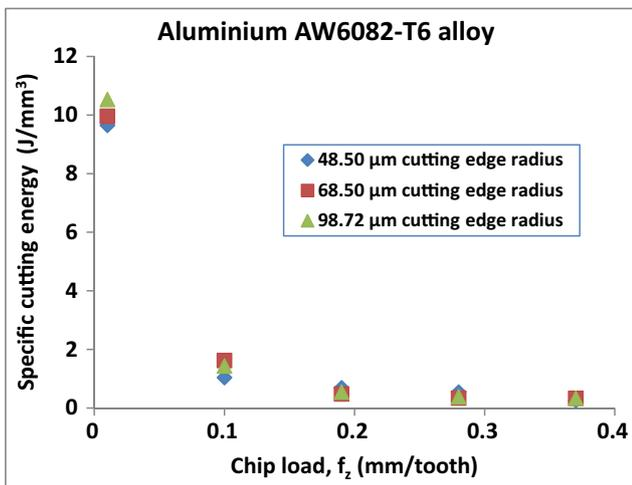
**Fig. 6** Variation of specific cutting energy with chip load during side milling of aluminium AW6082-T6 alloy with different cutting edge radii
