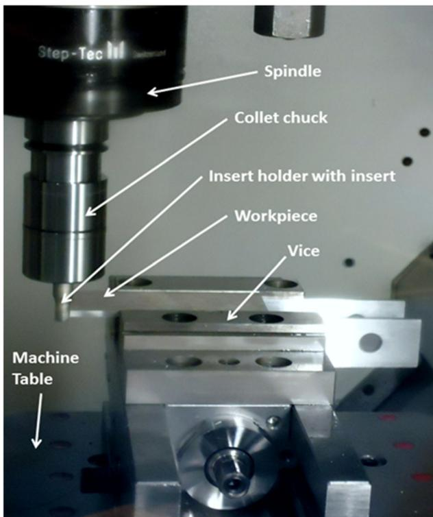
**Fig. 2** Setup for side milling operation on Mikron HSM 400 milling machining centre
