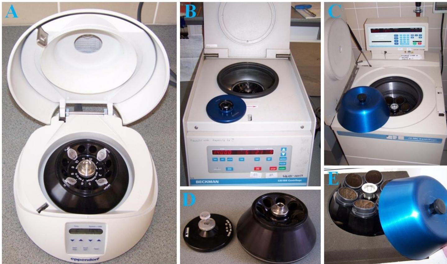
A, Bench-top Eppendorf centrifuge with samples arranged symmetrically around the axis of the rotor. B, Semi-preparative, refrigerated centrifuge with a rotor for Eppendorf tubes. C, Preparative, refrigerated centrifuge with a rotor for the handling of volumes up to 6 litres. D, Semi-preparative rotor with lid. E, Preparative rotor with lid.
