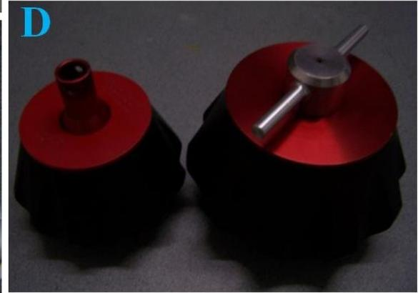
A, Micro-ultracentrifuge. B, Rotors compatible with the micro-ultracentrifuge. C, Semi-preparative ultracentrifuge. D, Rotors compatible with the semi-preparative ultracentrifuge.
